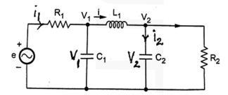
8. a) Find the pulse transfer function for the error sampled system shown in figure.
